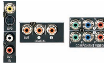
Figure 22 – DVD AV, Digital Audio and Component Video Inputs
